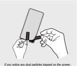
stick a dust remover tab on the screen protector, gently lift the screen protector and remove the dust using a second dust remover tab. Repeat **step 9** to complete the application.
