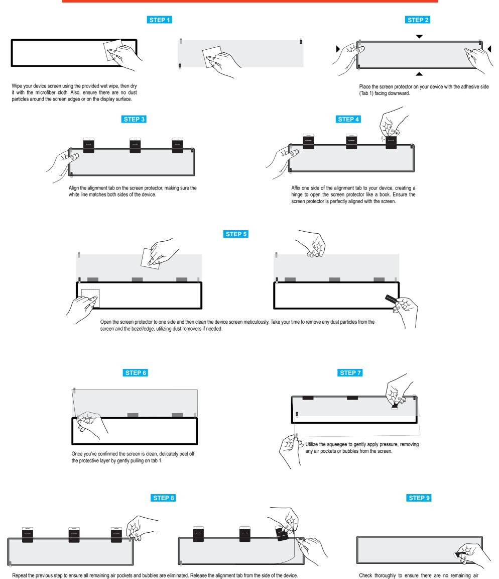
Repeat the previous step to ensure all remaining air pockets and bubbles are eliminated. Release the alignment tab from the side of the device. With one hand, hold the screen and then peel off the top layer by pulling tab 2, which is the side facing the surface.
